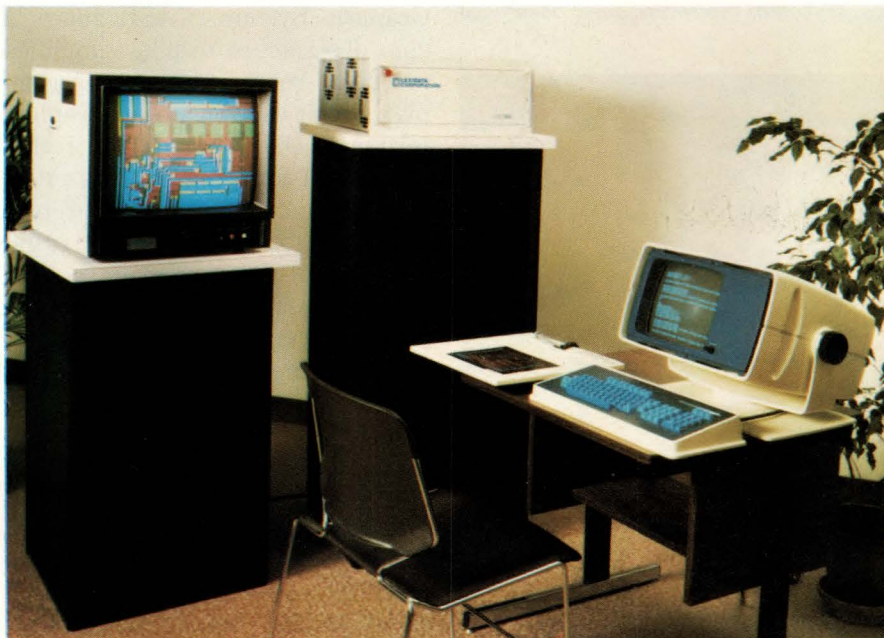
Color raster-type graphics terminals such as Lexidata's (left) are typical of the large, high-resolution displays available for CAD/CAM applications.
