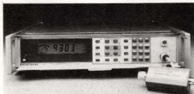
Autoranging, self calibration and computational capability highlight Model 9303. It measures 30 \mu V to 3V over a 100-kHz to 2-GHz range and displays voltage or relative stored reference values, decibels, watts, absolute and percent difference, or ratio.
