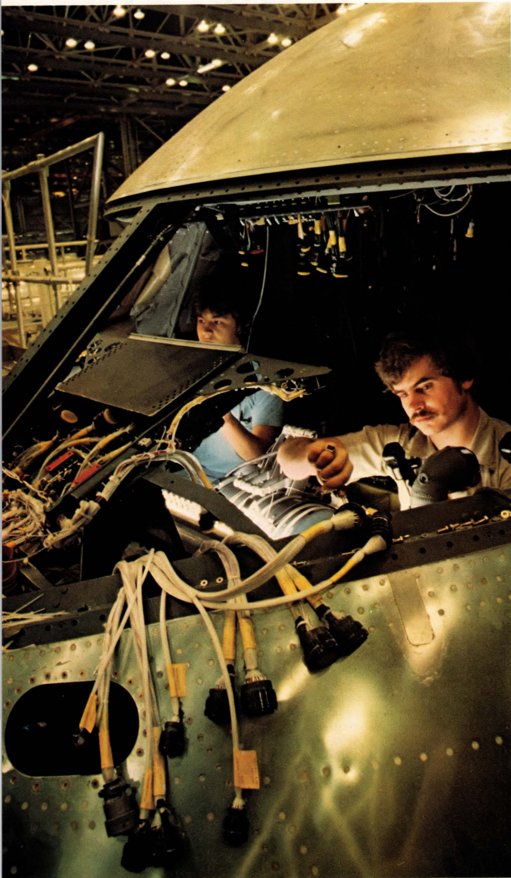
A Boeing 747 jumbo jet contains two tons of copper wire: 49,000 separate segments. Keeping track of the details of this massive electrical system requires the services of a large IBM computer.
